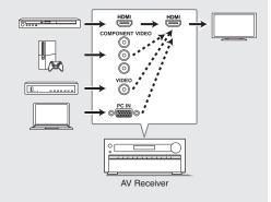
\* If multiple video signal inputs are put into one input system, the output will be made in the order of HDMI, component video, and composite video.
